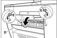
20 5 Troubleshooting 3 Hold both sides of paper and carefully pull the bottom edge of paper out of the machine.
