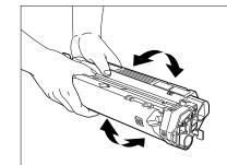
3. Hold the cartridge. Break the tab (A) and pull out the seal (B) completely.
