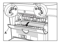
**4** Hold both sides of the jammed paper and carefully move it inward, then gently pull it out.
