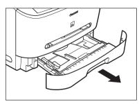
**3** While holding the lock release lever on the paper guide at the rear of the cassette, slide the paper guide to the mark indicating the desired paper size.
