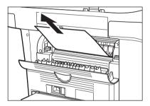
If the jammed paper is badly folded, similar to the folds of an accordion, ease the jammed paper loose and then pull it out of the machine.
