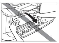
• Do not pull the jammed paper upward; the toner on the paper will stain the machine and cause a permanent reduction in print quality.
