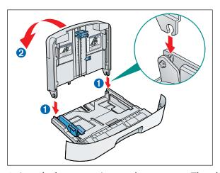
3 Attach the extension to the cassette. The slots 1 are keyed and must be inserted at a 90° angle. Once inserted, fold the extension as shown 2.
