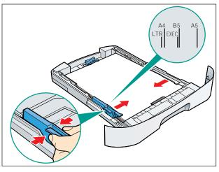
**6** Pinch and slide the side paper end guides to match the size of paper.
