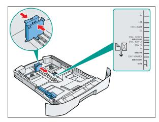
**4** Pinch and slide the rear paper end guide to match the size of paper.
