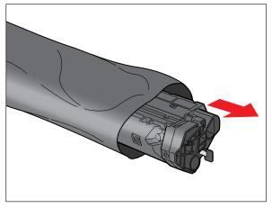
Remove the cartridge from the bag. Keep the bag in a safe place for future use.
