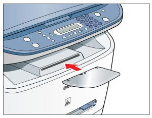
1 Insert the output tray into the front slot on the machine.
