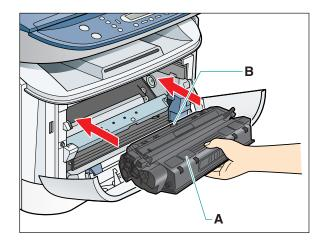
Hold the cartridge so that the instructions (**A**) and the arrow (**B**) are facing up, and insert it in the machine horizontally as far as it will go.
