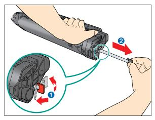
3 Hold the cartridge on a flat stable surface with one hand, and break the tab 1 and pull out the seal 2 completely with the other hand.
