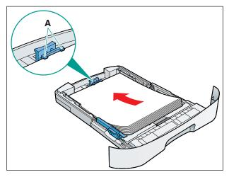
**5** Load the paper into the cassette. Make sure the paper stack sits below the hooks (**A**).
