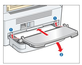
9 Insert the tabs on the extension cover into the slots 1 on the back of the machine, and carefully lower the cover 2 until it sits on the cassette extension beneath it.
