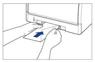
When the envelope is loaded, it is sent into the slot a little.
