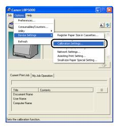
3 Select the [Use Periodical Calibration Timer] check box in the [Calibration Settings] dialog box, then specify the time to perform calibration in [Time].
