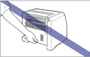
• The front portion of the printer (A) is relatively heavy. Be careful not to get off-balanced when lifting the printer. If you do so, you may drop the printer, resulting in personal injury.
