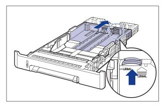
• While holding the lock release lever of the side paper guides, slide the guides to the mark for the size of the paper to be loaded.
