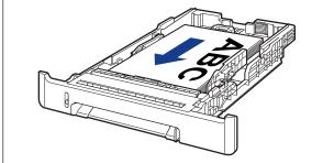
4 While holding the lock release lever of the side paper guides, slide the guides to the mark for the size of the loaded paper.
