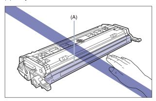
7 Hold the toner cartridge properly with the arrowed side facing up as shown in the figure.
