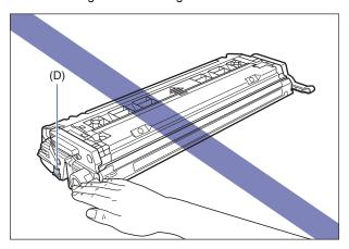
• When handling a toner cartridge, hold it properly as shown in the figure and handle it with the arrowed side facing up. Do not place it vertically or upside-down.
