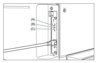
If the network board is not working properly, turn the printer OFF, and then check the LAN cable connection, hub performance, and network board installation.
