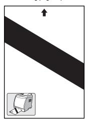
5 Load the cleaning page in the manual feed slot with the printed side facing up.
