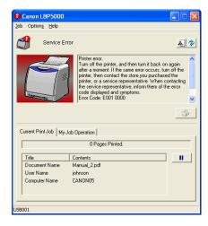
If the service call appears, cycle the power of the printer using the following procedure. This may clear the message.
