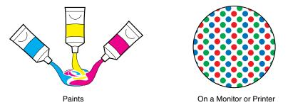
On the computer display, various colors are reproduced by the intensity of three red, green, and blue dots.
