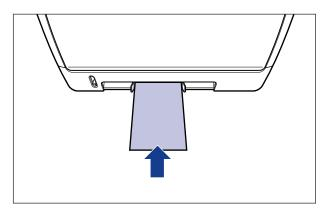
Adjust the paper guides to the width of the loaded Index Card size media as shown in the figure.
