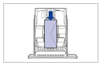
• When printing envelopes of the Envelope B5 size, close the flaps and load them so that the printing side is facing up and the envelopes are printed from the top (the edge with the flap).
