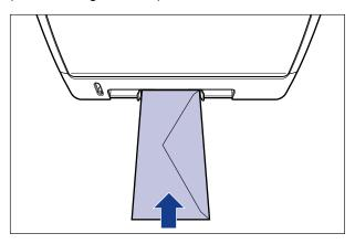
When printing an envelope of the Envelope B5 size, close the flap and load it so that the printing side is facing down and the envelope is printed from the top (the edge with the flap).
