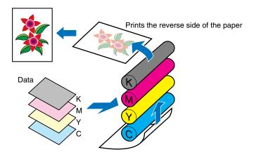
The data for all four colors is then transferred onto paper, and the paper passes through the fixing unit and is output.
