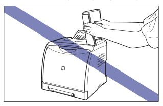
• Be sure not to open the covers on the printer during printing. This may result in damage to the printer.
