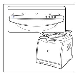
When the  $\triangle$  (Alarm) indicator is on, a service error is occurring. In this case, see "Service Call Display," on p. 7-14.
