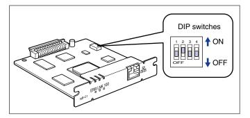
5 Insert the network board into the expansion slot.
