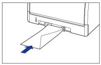
• When printing envelopes of the Envelope B5 size, close the flaps and load them so that the envelopes are printed from the top (the edge with the flap).
