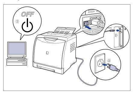
Remove all the interface cables and the power cord from the printer.
