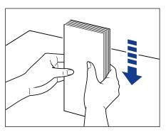
5 Load the envelopes so that the edge of the media is aligned with the front side of the paper cassette.
