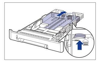
3 Load the paper so that the edge of the paper is aligned with the front side of the paper cassette.
