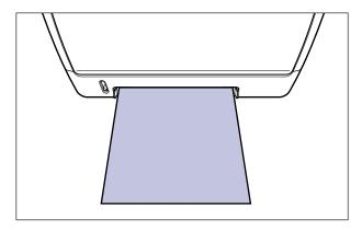
1 Adjust the paper guides to the width of the loaded paper as shown in the figure.
