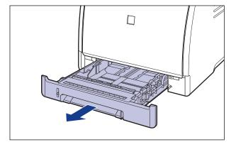
If the paper feeder is installed, pull out the paper cassette of the paper feeder also.
