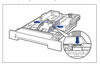
4 While holding the lock release lever of the rear paper guide, slide the paper guide.
