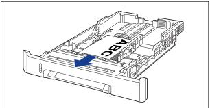
4 While holding the lock release lever of the side paper guides, slide the guides to the mark for the size of the loaded Index Card size media.
