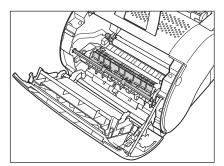
• Never touch the high-voltage contact points inside the front cover. This could damage the printer.
