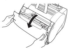
Remove the cartridge by grasping the cartridge's handle and lifting it out of the printer.
