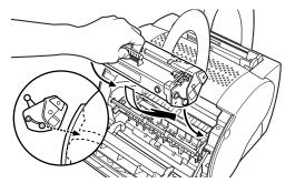
8 Close the front cover immediately after inserting a cartridge.
