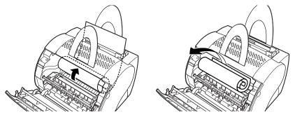
Do not pull the paper upwards from the paper input slot, as this may damage the printer. Gently pull the paper out of the printer.
