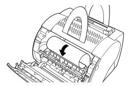
Gently pull the rolled up paper out of the printer.
