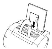
**2** Adjust the paper guides to the sheet of paper.
