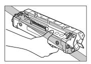
Hold the cartridge, then gently rock it from side to side five or six times to distribute the toner evenly inside the cartridge.
