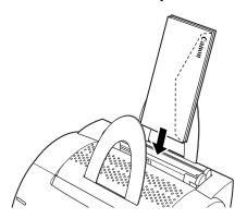
**2** Adjust the paper guides to the width of the stack of envelopes.
