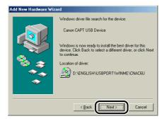
Installation of the USB class driver starts.
