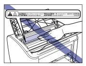
Keep your hands or clothing away from the roller in the output area after removing jammed paper completely. Even if the printer is not printing, sudden rotation of the roller may catch your hands or clothing, resulting in personal injury.
