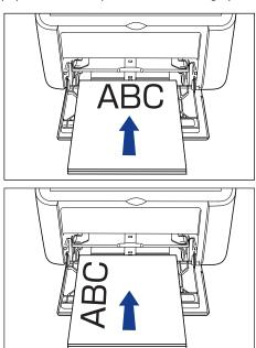
Slide the paper guides to fit both sides of the stack.
