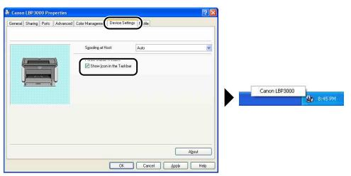
The Printer Status Window is automatically displayed during printing and if an error occurs. If [Display Printer Status Window] is not set to [When Starting Printing] in the [Preferences] of the [Options] menu in the Printer Status Window, the Printer Status Window will not be displayed during printing. (See "Setting Preferences," on p. 4-64.)
