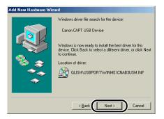
Installation of the USB class driver starts.
