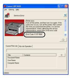
**3** Turn the printer and computer off ①, remove the USB cable ②, and disconnect the power plug from the power outlet 3.
