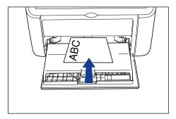
3 Slide the paper guides to fit both sides of the index card.
