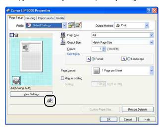
Check the [Show Icon in the Taskbar] box in the [Configuration]/[Device Settings] sheet in the [Printer Properties] dialog box. A Printer Status Window icon is then shown in the Windows Taskbar, and you can click on this icon, then click [Canon LBP3000] to open the window.
