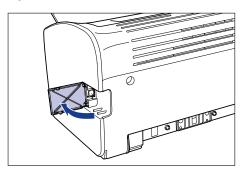
3 Connect the B-type (square) end of the USB cable to the USB connector on the rear side of the printer, then close the USB cover.
