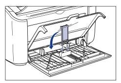
☐ Slide the rear paper guide ① to align the small paper guide with the paper, and close the tray cover ②.
