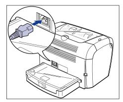
**3** Plug the power plug into the AC power outlet.
