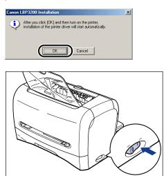
Installation of the printer driver and the USB class driver will start automatically.
