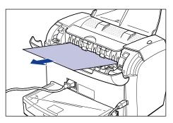
**8** Slowly pull out the paper jammed in the face-down delivery area in the direction of the arrow.
