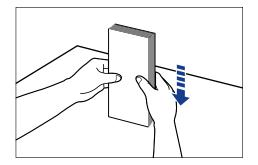
**6** Load the envelopes so that the rear edges of the envelopes touch the paper guide.
