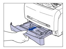
**2** While holding the lock release lever on the paper guide at the rear of the cassette, slide the paper guide to the mark indicating the desired paper size.
